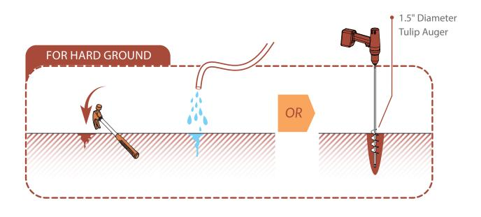
FOR HARDER GROUND If your ground is really hard, you may need to dig a hole large enough to accommodate one post from each panel - Approximately 8" in diameter and 12" deep. Backfill and compact the dirt. = 8 in. 12 in.
